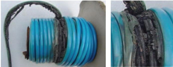
Picture 1: Results of overheating in cable. (This may not be evident until the cable is unreeled).
